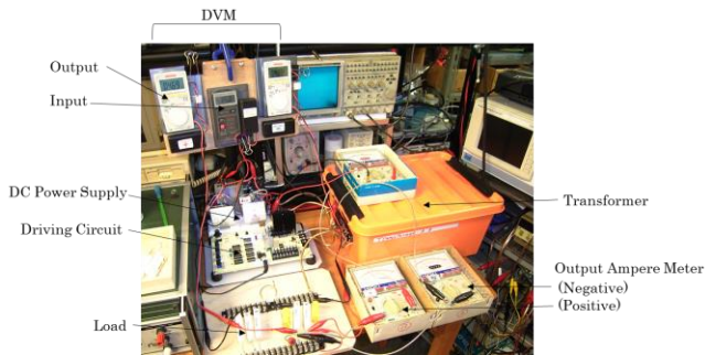
Figure 2 . Overview of the whole experimental setup
