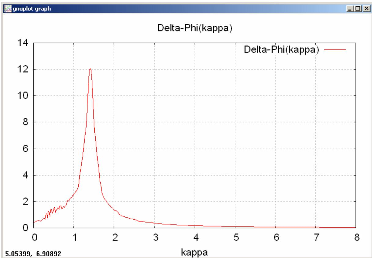
Fig. 4. Model 1: Amplitude resonance curve  $\Phi_{\max}(\kappa)$
