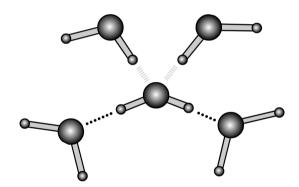
Figure 11.4: The water lattice. Each water molecule acts to accept and donate four hydrogen bonds. The subunit  $O-H \cdots O$  is essentially linear. Reproduced from Robitaille [75], with permission.
