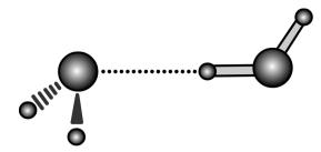
Figure 11.5: Schematic representation of the trans-linear water dimer. The subunit  $O-H \cdots O$  is essentially linear. Reproduced from Robitaille [75], with permission.
