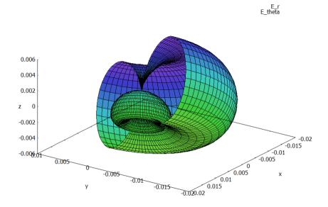
Figure 8.36: Components  $E_r$  (outer) and  $E_{\theta}$  (inner) of electric field for the magnetostatic current loop, spherical distribution.
