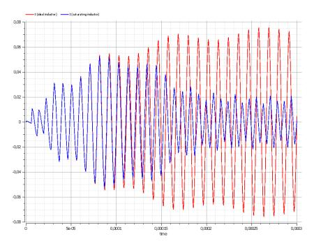
Figure 5: Current of an ideal inductor (red) and saturated inductor (blue) for an ordinary serial resonance circuit.
