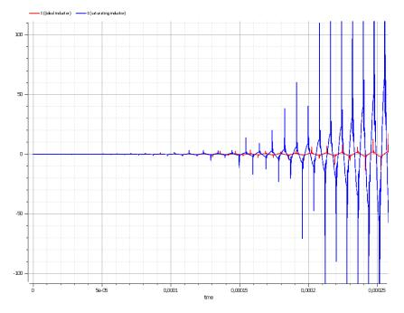
Figure 7: Current of an ideal inductor (red) and saturated inductor (blue) for the parametric resonance circuit.
