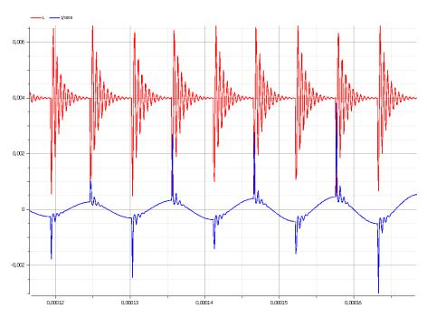
Figure 3: Variable inductance L and current I in an enlarged time slot.
