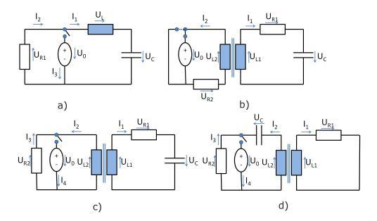
Figure 8: Variants of the parametric oscillator circuit. a) source position modified, b) inductive coupling for Fig. 1a, c) inductive coupling for (a), d) oscillator completely in primary circuit.
